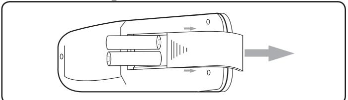
1. To install the batteries, first remove the battery compartment lid from the back of the remote control.
